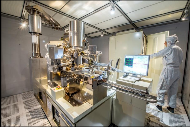
Electron Beam Lithography JEOL JBX6300FS (100 kV) Raith eLine, Raith eLine plus (< 30 kV)
