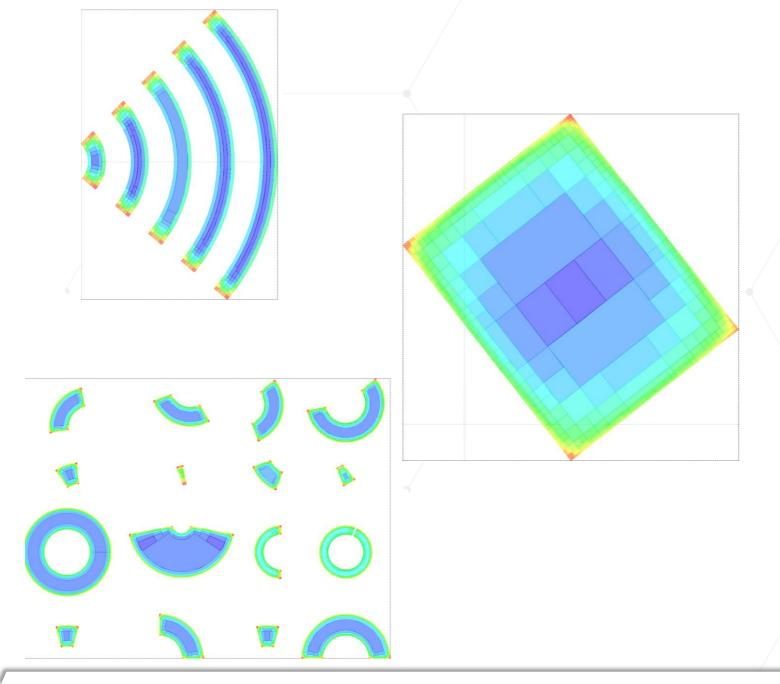
Generic element types like Circles / Arcs / Rotated Rectangles are maintained during fracturing. Dose fracturing of PEC will fracture e.g. ARC elements only into smaller ARC elements to improve the fracture quality.
