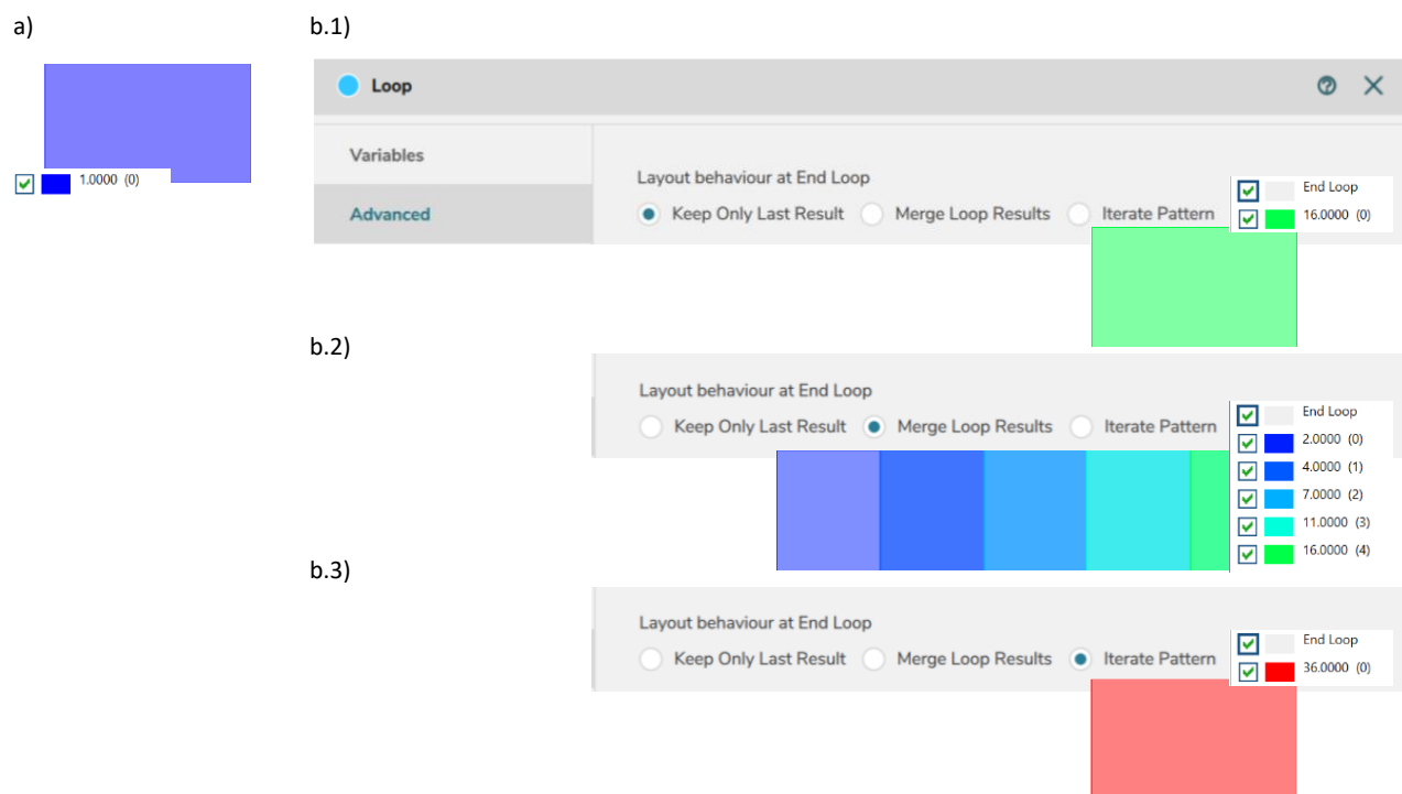
Figure 12. a) Layout that enters to the loop module with a dose of 1, b) result of the layout using different ending loop behaviour.
